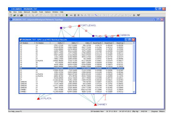
The Local Horizon NEU residuals help in the detection of receiver centering and height measurement errors over the AT or TO stations. To compute the Local Horizon NEU residual for each baseline, the GPS XYZ residuals are transformed to Local Horizon NEU residuals based on the mean geodetic position for each AT and TO station pair (i.e., at the midpoint of the GPS vector).
