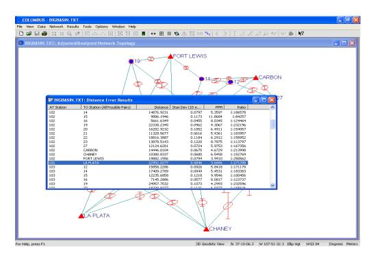
In the screen above, the distance error from Station 102 to Station LA PLATA is highlighted. The standard deviation has been scaled to the 95 percent confidence level by the expansion factor 1.95937 (shown in the Standard Deviation column). The distance represents the adjusted chord distance between the two
