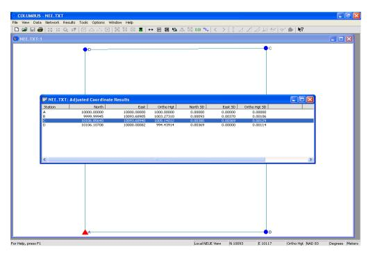
In the screen above, the adjusted north, east and orthometric height for Station C is highlighted (from sample project NEE.TXT).
