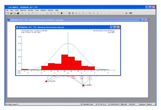
The figure above represents the histogram of standardized residuals for our 3D Geodetic network, BIGBASIN.TXT. As more observations are added to the network, the distribution will generally approach normality (unless there is a problem in the network). The x-axis of the diagram contains two sets of values:
