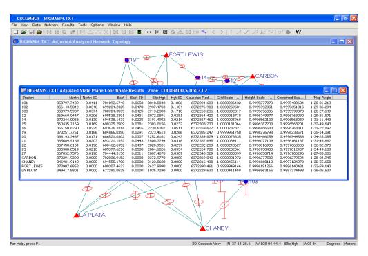
For each station, the adjusted grid north, grid east, and height are shown along with their standard deviation. Also shown is the gaussian radius, grid scale factor, height scale factor, combined scale factor, and the grid mapping angle.
