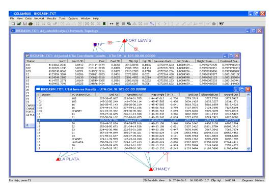
The results for each UTM inverse include the grid azimuth, geodetic azimuth, mapping angle, (t-T) correction, grid distance, ellipsoidal distance, and the ground distance.
